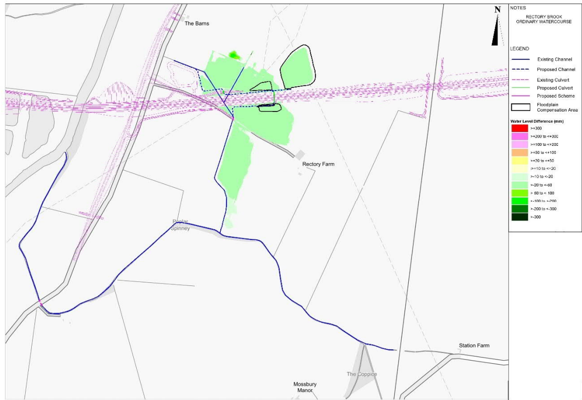
Figure 11-12 Flood depth differences when inflow -20%, during a 1% AEP + 65% CCA event, as reported in Table 11-5.
