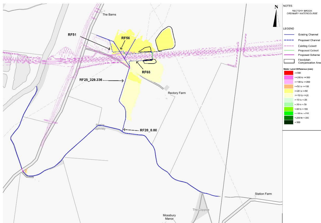
Figure 11-11: Flood depth differences when inflow +20%, during a 1% AEP + 65% CCA, as reported in Table 11-5.
