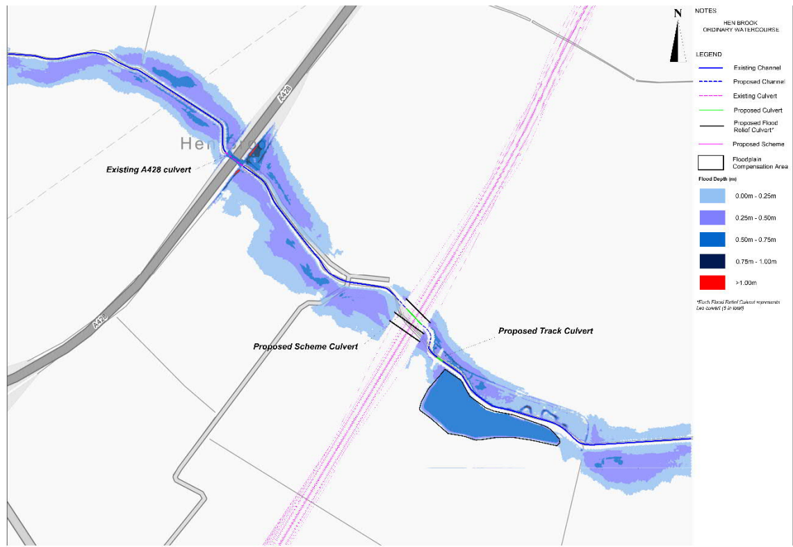
Figure 10-6: Proposed Maximum Flood Depth Map – 1% AEP + 65% CCA
