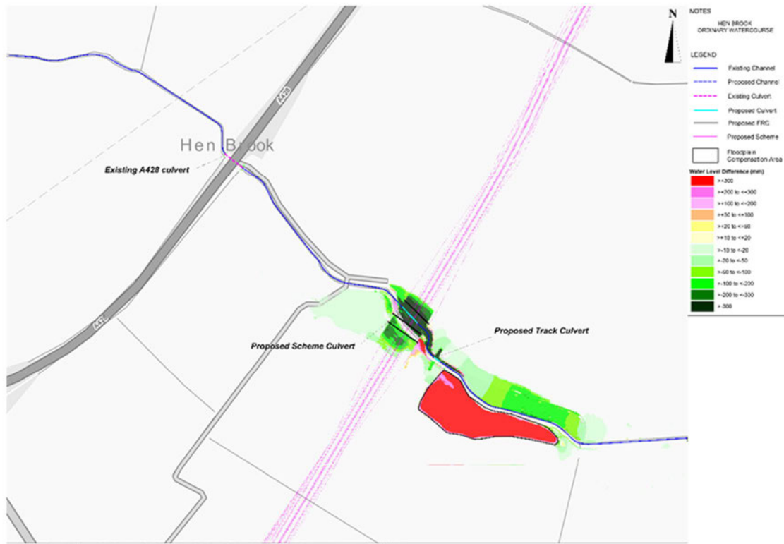
Figure 10-7: Depth Difference Map (Baseline vs Proposed) – 1% AEP + 65% CCA
